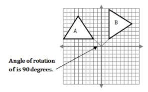
Draw a line from each point to the center of rotation, in this case it's the origin. Measure  $90^{\,0}$  from the object using the protacter and make sure the base line of the proctacter is on the same line as the line from the point of the object to the center. The 0 mark should start from the object.
