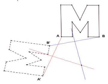
Justify your construction by measuring angles  $\angle APA'$  and  $\angle BPB'$ . Did you obtain the same measure? The angle between is the angle of rotation. The zero mark of protector should be on the object to give you the direction of rotation.
