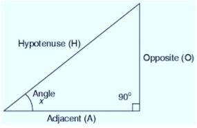
In the figure above adjacent length is 4 cm and Angle  $x = 36^{\circ}$ . Calculate the opposite length.
