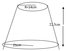
The diagram represent a solid frustum with base radius 21cm and top radius 14cm. The frustum is 22.5cm high and is made of a metal whose density is 3g/cm3 = 22/7.
