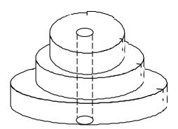
17. A right conical frustum of base radius 7 cm and top radius 3.5 cm and height 6 cm is stuck onto a cylinder of base radius 7 cm and height 5 cm which is further attached to form a closed solid as shown below.
