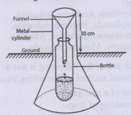
The instrument is used to measure the amount of water
